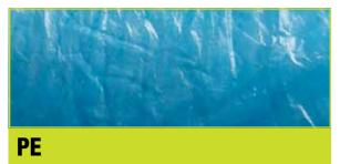
Polyethylene (PE) is a thermoplastic polymer and one of the most widely produced plastics in the world. Being a thermoplastic means PE can be heated to its melting point more than once without significant degradation, meaning products manufactured out of this material are easily recyclable. PE provides great short term liquid barrier protection but lacks breathability, resembling more of a plastic than a cloth.
