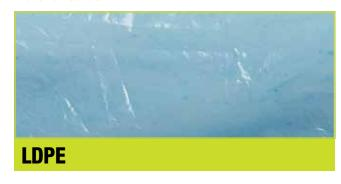
Low Density Polyethylene (LDPE) is the low density version of PE. Similar to PE, LDPE has excellent resistance to water, moisture and most organic solvents and chemicals. LDPE has high ductility but low tensile strength, which is evident by its propensity to stretch. LDPE is highly flexible and perfect for protective garments which have a short term requirement.
