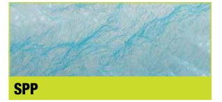
Spunbonded Polypropylene is a lightweight and breathable fabric offering exceptional protection against non-hazardous dry particles. It is an economical solution to protecting workers in dry, dirty environments.
