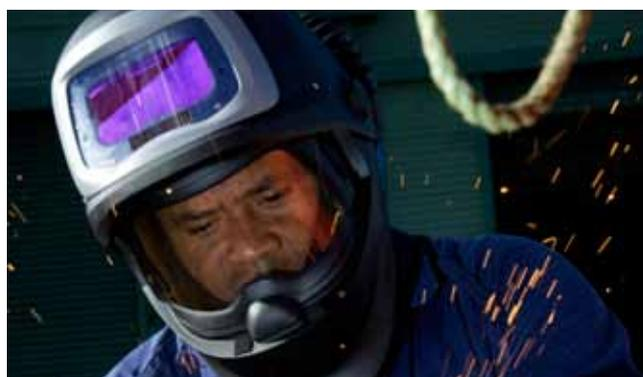
A spark and spatter-resistant head cover is included as standard in all 9100 FX & FX Air series welding helmets. An optional extended-length head cover and ear/neck protection are available as accessories.
