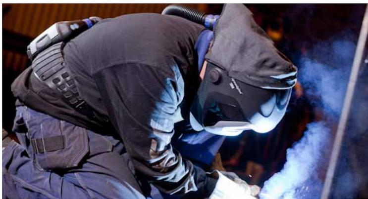
**Extended protection:** A flame-resistant headcover (used in this application) and ear/neck protection are available as accessories to all Speedglas 9100 series welding helmets.
